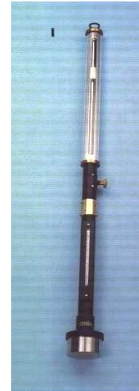
Pressure or atmospheric pressure is a measure of the force being exerted by air molecules at a particular location. A barometer is used to determine the pressure and the units used are millibars (mb). The standard type of barometer used by meteorologists is referred to as the **Kew Pattern Barometer**.
