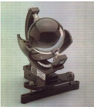
The number of hours of sunshine per day is also important in some sectors for example the construction industry. This parameter is measured by a **Campbell - Stokes Pattern Sunshine Recorder**.
