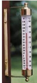
The **thermometer** with which we are all familiar is used to measure air temperature. The four main types are maximum, minimum, wet and dry bulb. Temperature is measured in degrees Celsius ( $^{\circ}\text{C}$ ).
