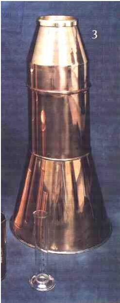
The rain gauge gives the total recorded rainfall for a 24 hour period while the data logger records the time of occurrence as well as the amount. Rainfall is measured in millimeters (mm).
