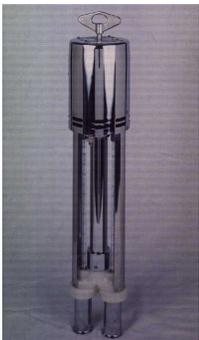
The **aspirated hygrometer** is used to measure both wet and dry temperatures, which in turn are used to determine humidity.
